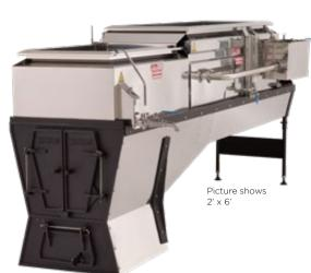
A high efficiency evaporator with a 7" deep raised flue pan but assembled with basic plumbing connections (similar to the Junior model). There is only one pan in the front with two partitions (three compartments) going width wise and return connection boxes on opposite corners. This model will give you the same boiling rate per hour compare to our Storm model but for less money.
