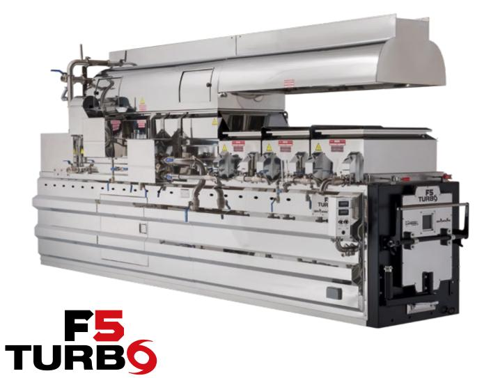
The Force 5 TURBO is the fusion between the best combustion controlled wood arch and the Lapierre-Waterloo-Small designed fire tube double pass Turbo pan. A combination that makes evaporating with wood even more efficient and economical!
